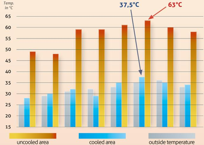
At an outside temperature of 35°C, the uncooled surface reached a temperature of over **63°C**! The water-cooled area, on the other hand, was a cool **37.5°C**. That's just above the outside temperature and that for several days!
